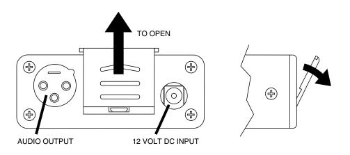
Swing the door open and take note of the polarity marked inside showing the location of the positive (+) and negative (-) terminals. Insert the battery and close the cover by pressing in and across, reversing the opening procedure outlined above. Note that the battery door will NOT close if the battery is inserted incorrectly, since the terminals will hit a protective polarity barrier. Do not force the battery in.
